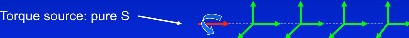
Min / max source-receiver offset: 1 m / 4 m
