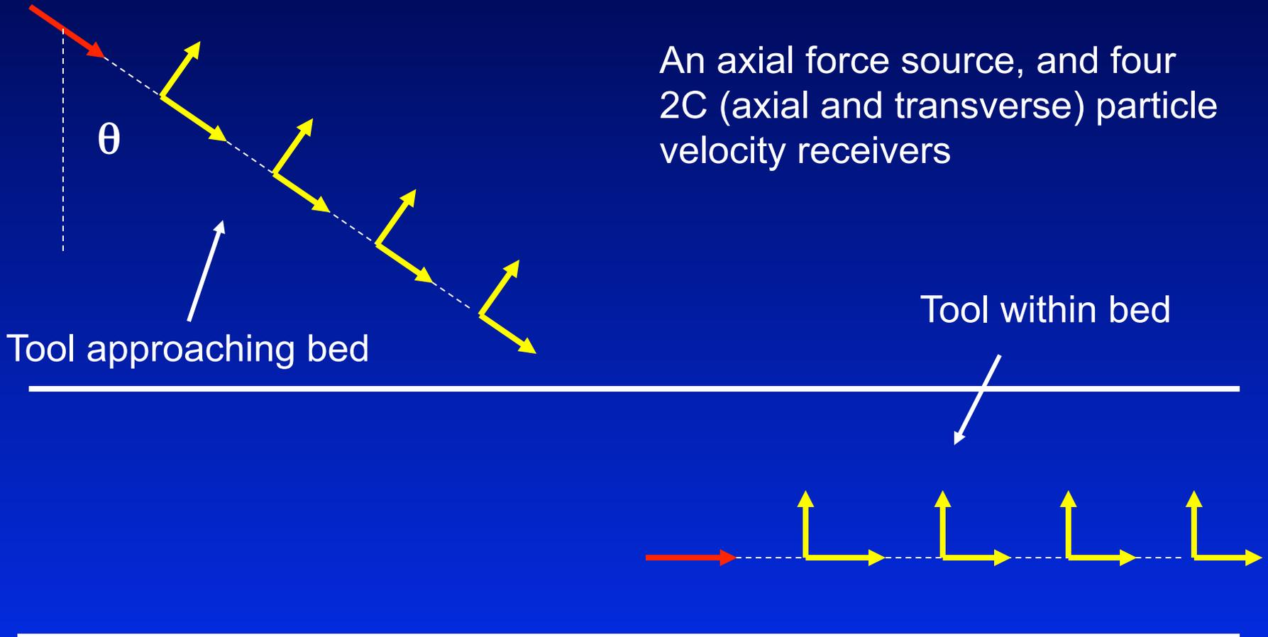
Min / max source-receiver offset: 1 m / 4 m
