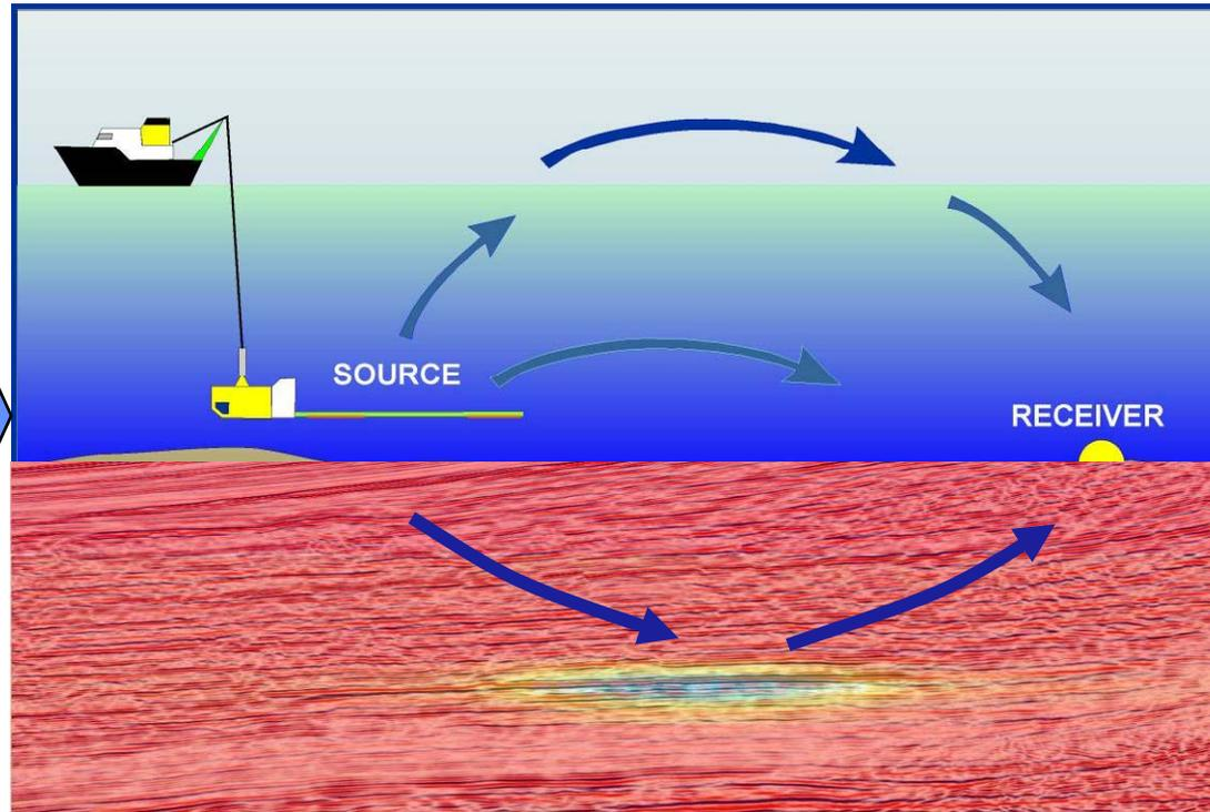
Receiver arrays detect changes in the earth's response to this signal.
