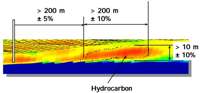
Figure 1: Illustration of the DeepLook consortium objective to map a reservoir up to 200 m away from the wellbore including its fluid properties and fluid movements (After DeepLook website [www.DeepLook.com](http://www.DeepLook.com)).
