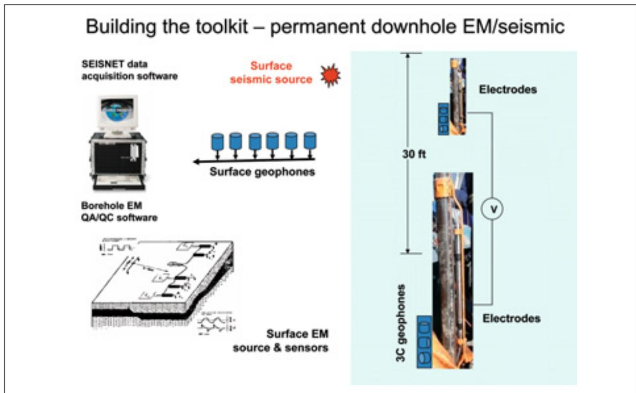
**Figure 2** Generalized schematic showing the linkages of borehole and surface measurements of EM and seismic. Recording in the borehole provides optimal resolution while recording at the surface provides areal coverage. System integration is the key.
