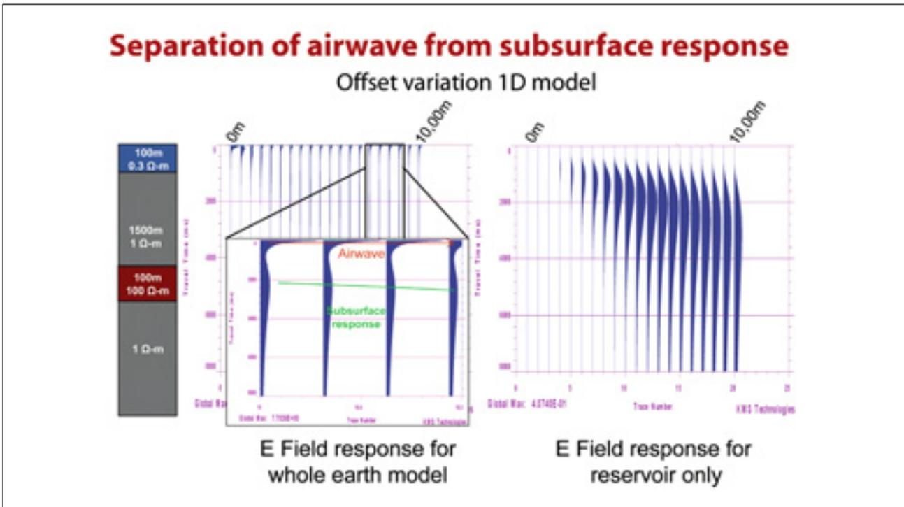
**Figure 3** Time domain 1D forward model for a typical reservoir in shallow water. Transients are treated like seismic traces and create a common receiver gather. The airwave phenomena can be shown to separate from the subsurface response as a function of time and offset in shallow water.
