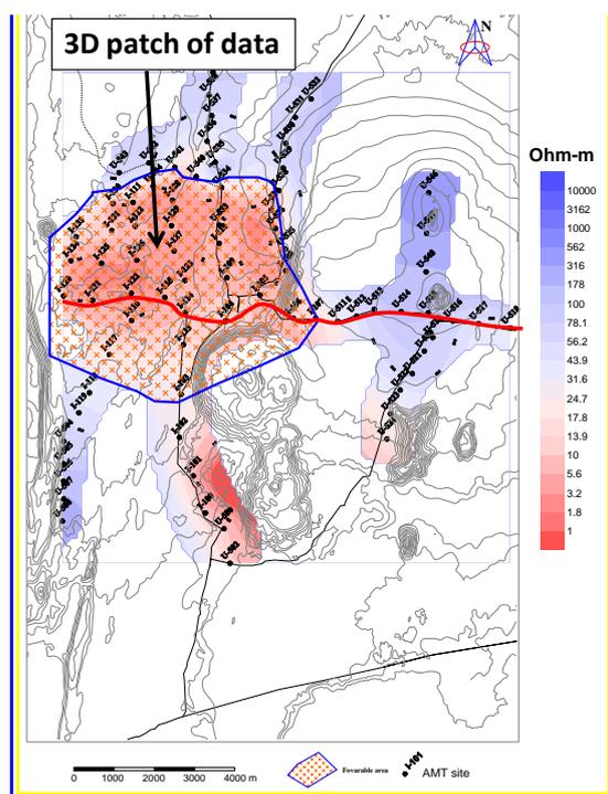
Figure 1. Map of survey area with site locations. Section 04 is highlighted in red. Inversion results from a depth of 500 m are overlain and describe the aerial extent of the upper conductive zone.
