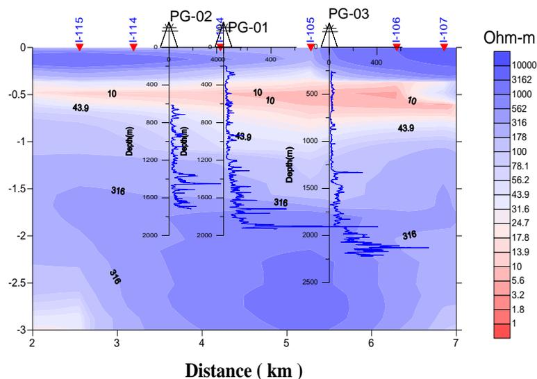
Figure 4. Expanded view of well ties along section 04. Note the strong correlation between borehole resistivity measurements and the inversion result
