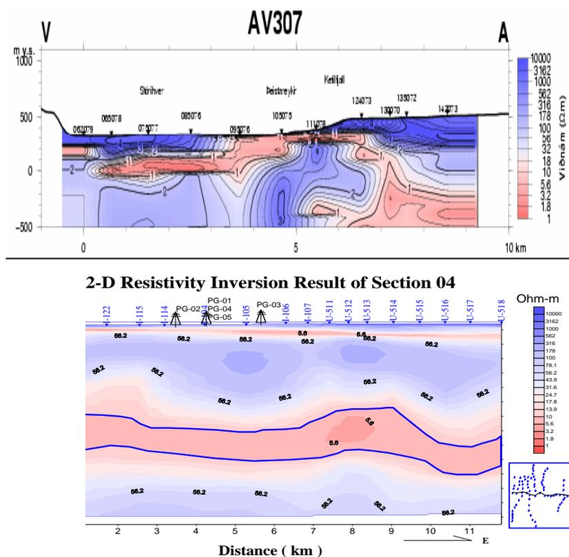
Figure 3. Top: TEM inversion result of profile 307 (from the ISOR report provided by the client); bottom: 2-D deep MT inversion section 04 shows the striking conductor in depth around 7 km. Location and orientation of the profile is show on the right map insert.
