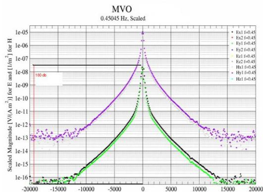
Figure 1: Magnitudes as a function of offset, acquired at a frequency of 0.4545 Hz. The green and black graphs represent the electric fields and the purple the magnetic fields. The data were acquired in deep water.
