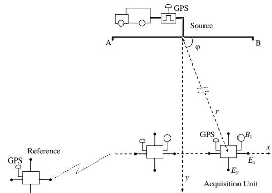
Figure 1 Array TEM survey setup
