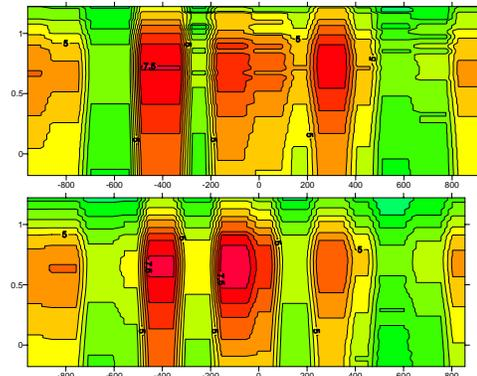
Figure 6 Cross sections of apparent resistivity for survey line #12 observed in July (below) and in November (above)
