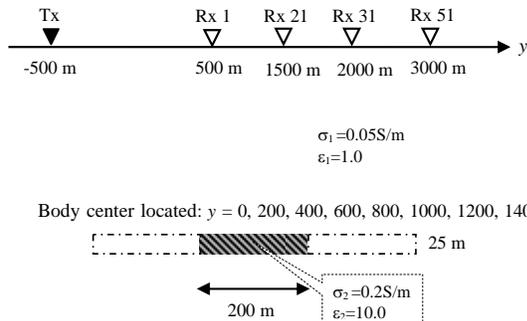
Figure 2 Model setup for water bearing reservoir
