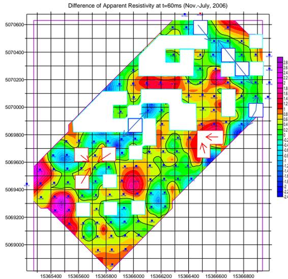
Figure 8. Apparent resistivity differences at  $t=60$ ms and qualitative inferred interpretation.
