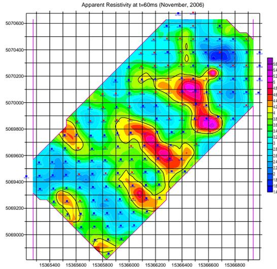
Figure 7. Apparent resistivity distribution at  $t=60$  ms from second survey (Nov. 2006)
