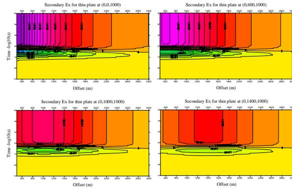
Figure 3 Secondary  $e_x$  responses for simulated water-bearing reservoir at  $y=0, 600, 1000, 1400$ m
