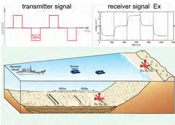
**Figure 1:** Schematic demonstration of the used broad side configuration and the form of the injected LOTEM signal as well as the observed signal of the electrical field.
