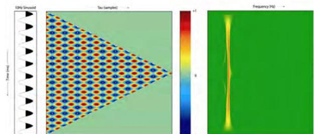
Figure 1: Spectral decomposition of a synthetic trace (far left) uses the discrete Wigner-Ville transform. Middle is the corresponding signals in the  $\tau$  domain, and right side shows the spectral amplitudes.
