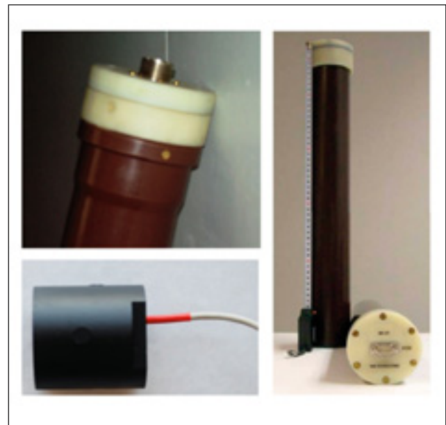
Figure 6 Marine induction coil magnetometer, MIC-121 (upper left), Land induction coil, LIC-120 (right), and flux-gate sensor (lower left).
