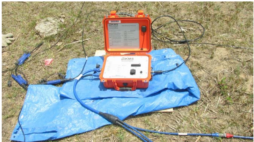
Figure 2: Field data acquisition with MT system.
