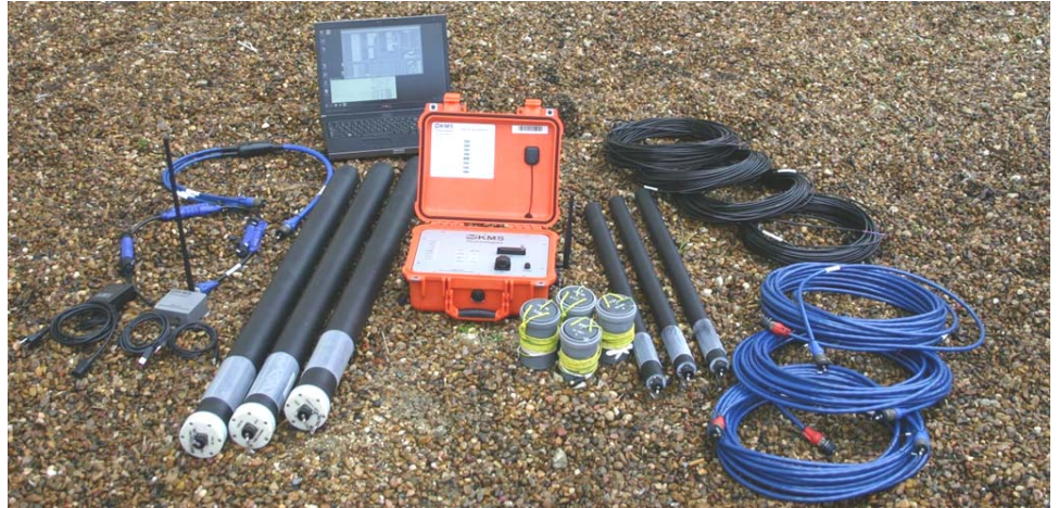
Figure 1: MT survey system: KMS-820 data acquisition unit, LEMI-118 and LEMI-120 induction coil magnetometers, LEMI-701 electrodes, wireless antenna.
