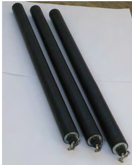
Figure 1: LEMI-118 induction coil magnetometer.
