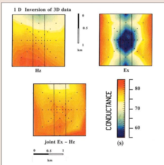
Figure 7. Plan view of the total conductances for the first and second layer across the dyke structure. The diagrams show the results after the 3D synthetic data were inverted with a 1D model. On the top are vertical magnetic fields and electric fields shown respectively. The bottom shows the joint inversion results of both (After Kriegshaeuser, 1992).
